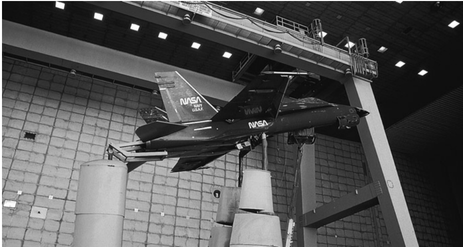
Wind tunnel test of an F-18 fighter plane model. Testing of models is imperative in the design of complex, expensive fluids-engineering devices. Such tests use the principles of dimensional analysis and modeling from this chapter. (Courtesy of Mark E. Gibson/Visuals Unlimited)
